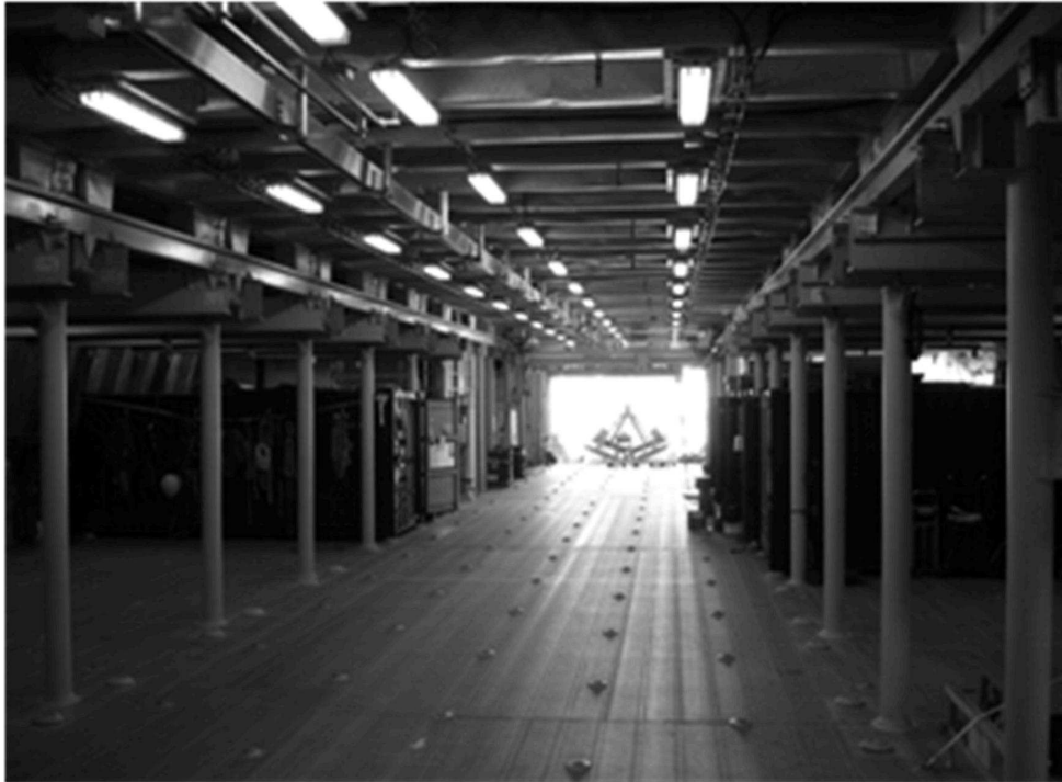
Figure 2. FSF-1 Sea Fighter mission bay. While an open space, the bay is occupied by large steel shipping containers as seen in this photo. 76x54mm (600 x 600 DPI)
