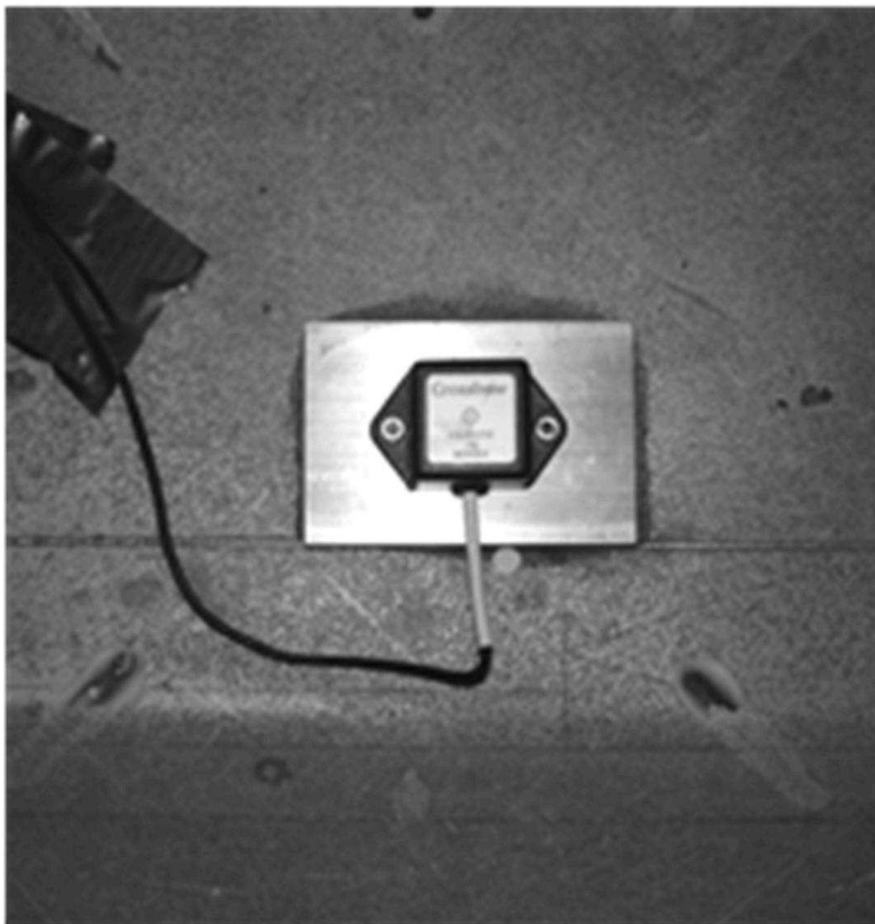
Figure 7. Details of the wireless sensor installation on Sea Fighter: (a) Four-pole Butterworth filter with Narada nodes for strain gauge de-noising; (b) Accelerometer bonded to mission bay deck by epoxy; (c) Wireless sensor within an enclosure with directional antenna installed in the mission bay. 46x48mm (600 x 600 DPI)
